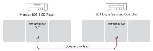
Connect the SpeakerLink output from the 808.3 to the SpeakerLink input on the 861, using a SpeakerLink lead.
