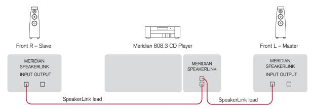
The 808.3 can be connected directly to Meridian DSP loudspeakers to create a complete compact stereo system, with volume and other preamplifier controls provided by the loudspeakers via the MSR+ or the front panel.
