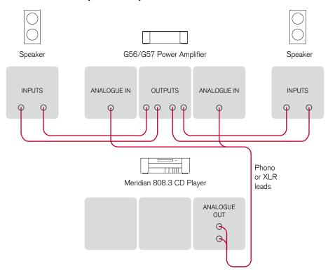
The 808.3 includes an integrated preamplifier, allowing you to connect it directly to a pair of analogue active loudspeakers, or to analogue passive loudspeakers via a power amplifier.
